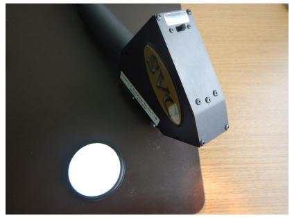
31. To collect a good reference, first align the business end of the probe on the Spectralon disc as shown below
