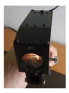
11. Install the plant probe battery to the plant probe. Again only hand tighten this connection.
