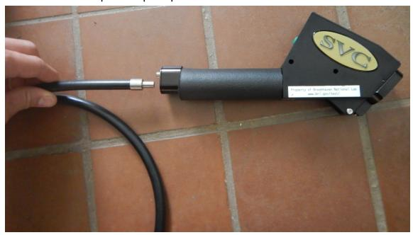
9. Confirm fiber optic is fully installed into the plant probe. To do this look into the business end of the probe for the end of the fiber optic which should be clearly visible behind the lens. See images below for proper fiber optic insertion. NOTE: blue tape on fiber also serves as a check for full fiber insertion
