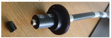
7. Insert fiber optic (FIBER1) into the spec body as shown below and hand tighten - **do not overtighten or tool tighten**. **NOTE:** you need to align the metal notch with the receptacle on the spectrometer body and then turn the collar counterclockwise to secure the fiber optic to the instrument.
