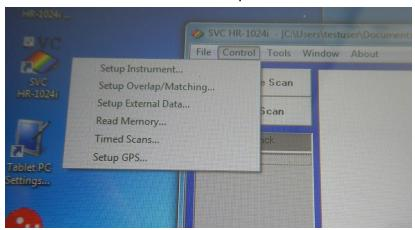
24. If this is the first time you are connecting to the instrument from a computer, you will need to set the correct comm port in the instrument setup. To do this go to the comm selection menu and scroll to the port number shown in step 20 (Default is 41)
