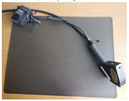
13. Turn on the plant probe lamp using the green power switch on the back. NOTE: Allow lamp to warm up for 10-15 minutes before use, however it is advised to turn this off during long periods of down time (i.e. longer than 20 minutes) to conserve battery and the life of the bulb
