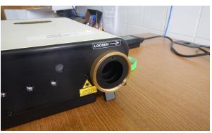
6. Remove protective rubber caps from fiber optic and place into the small ziploc bag in the spectrometer body pelican case
