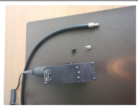
b. Insert fiber optic into plant probe
