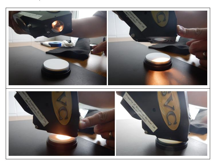
32. Once on the probe is in position, hit the "Reference" button
