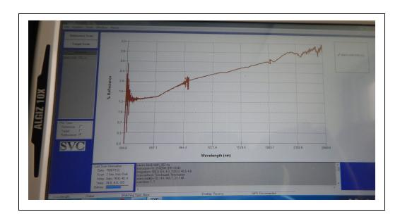
36. You can continue to collect spectra on your sample and the spectral curves will show on the screen together (seen below for the black cloth used behind the leaf samples)
