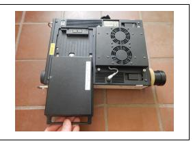
a. Or if possible you can use the spectrometer AC adapter. Insert this the same as you would a battery and then connect the power plug to the adapter and then to a wall socket or a power strip
